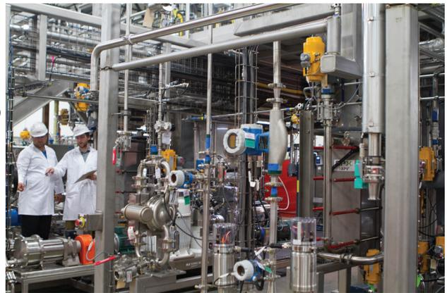
Both systems were designed to fit within limited shipping space, and for simple reconstruction upon arrival at their new location. Prior to shipping, the completed modular batch blending skids were disassembled, securely shipped under ISO container restraints, then successfully reassembled and installed on location. After successful start-up, EPIC demonstrated the new process in full production before fully handing off production to the client.
